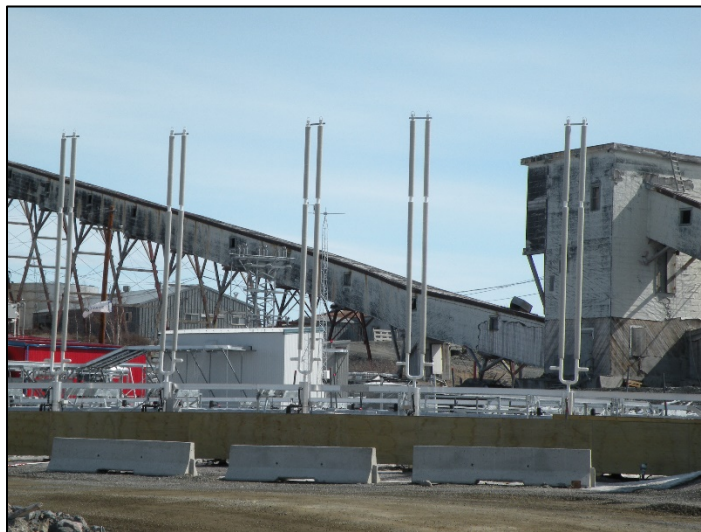
Fig. 2: Themosyphon freeze test plot, Giant Mine (credit: Arn Keeling)
